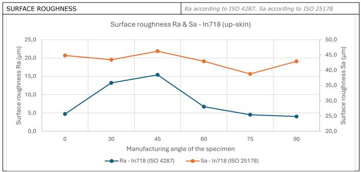
Manufacturing angle: 0° is the horizontal printing plane.
