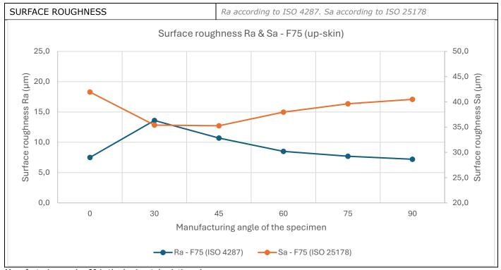
Manufacturing angle: 0° is the horizontal printing plane.
