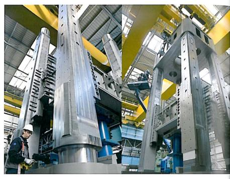
pre-tensioned case boxes, made of three, huge hollow-forged pieces.
