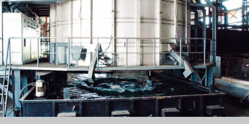
Aluminium electric-drop furnace which guarantees full immersion of batch charge within 5 seconds.
