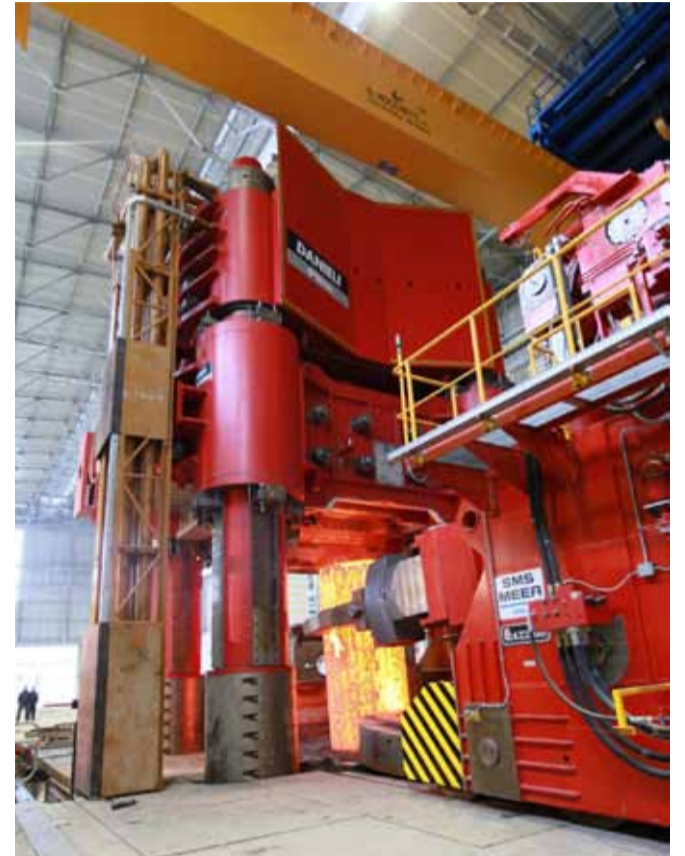
110 MN Open Die Press with 400 Tmt integrated manipulator
