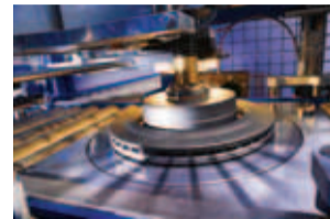
Vent inspection for brake discs.
