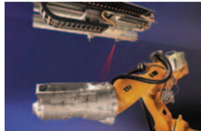
Gearbox housing presented by robot to light-section sensor.
