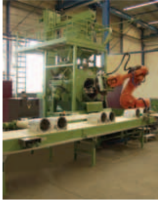
Rösler developed this highly efficient processing system for an automobile manufacturer to deburr and surface finish magnesium transmission housings.
